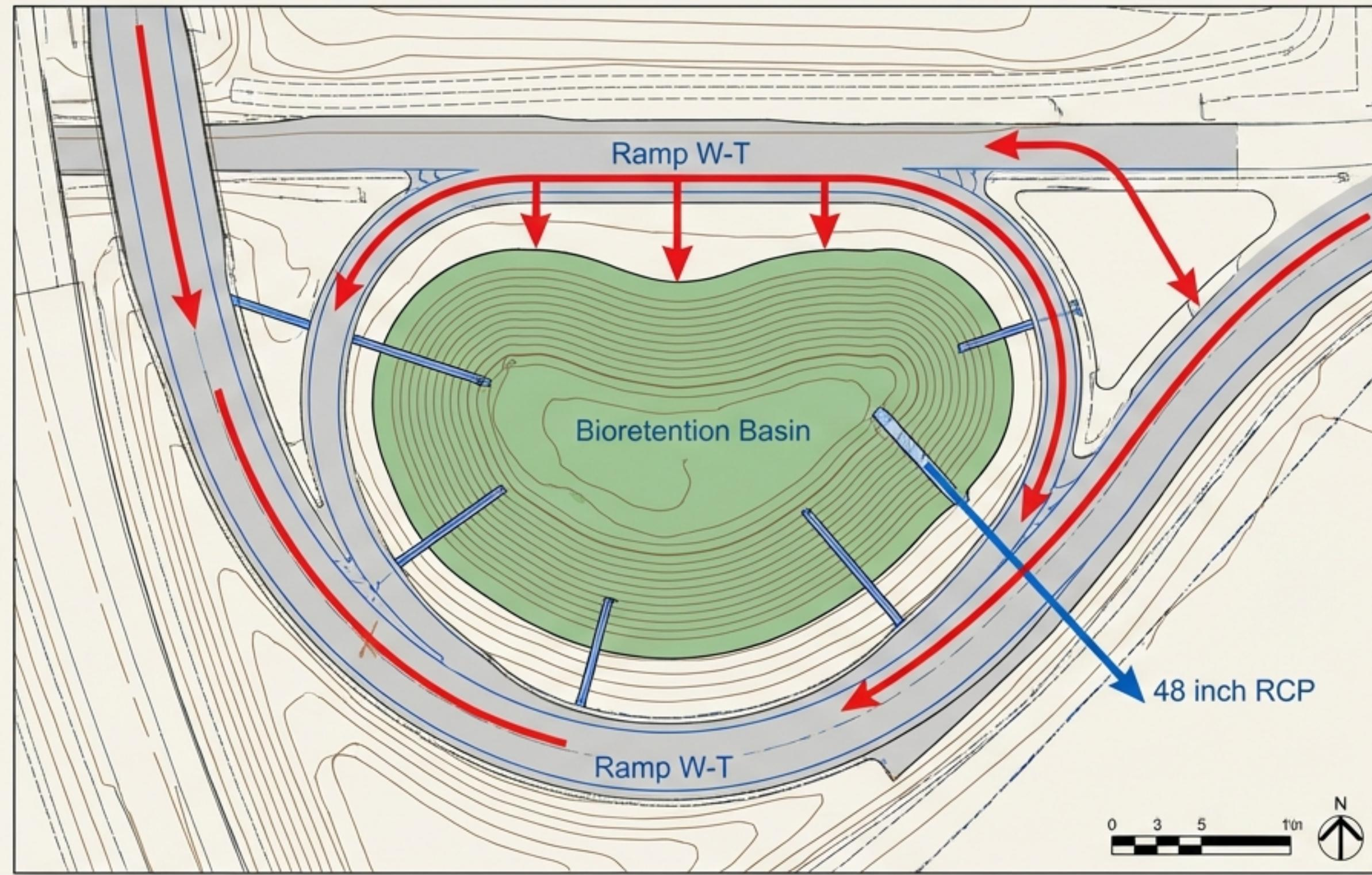
**Strategy:** Runoff from the new impervious ramps is directed into a specialized infiltration facility situated in the non-buildable loop space.
