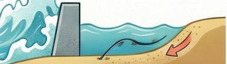
Blocks wave energy with static, strong walls, which can increase erosion elsewhere.
