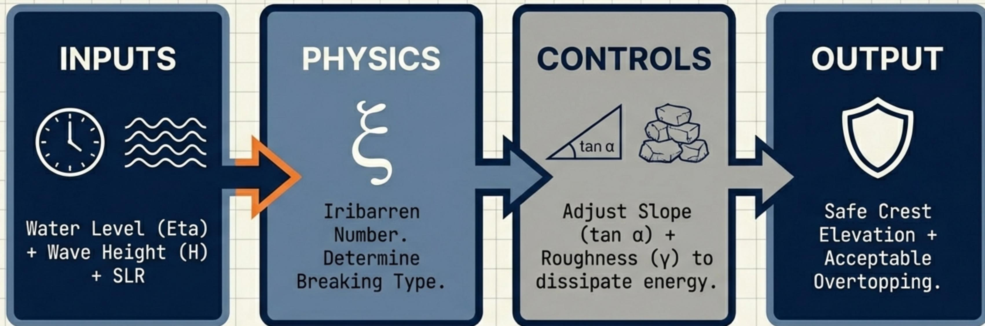
Hard structures resist force through mass and geometry. Success lies in accurate load prediction and energy dissipation.
