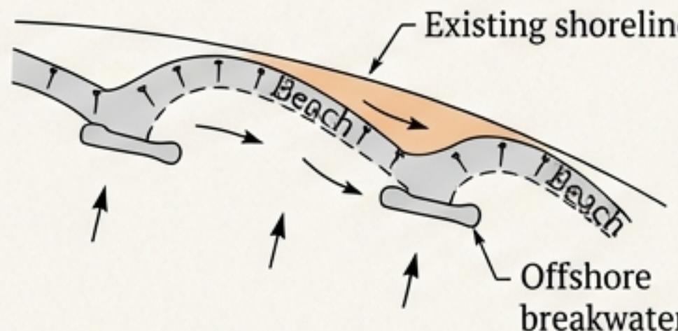
Parallel (Offshore). Reduces wave energy.
