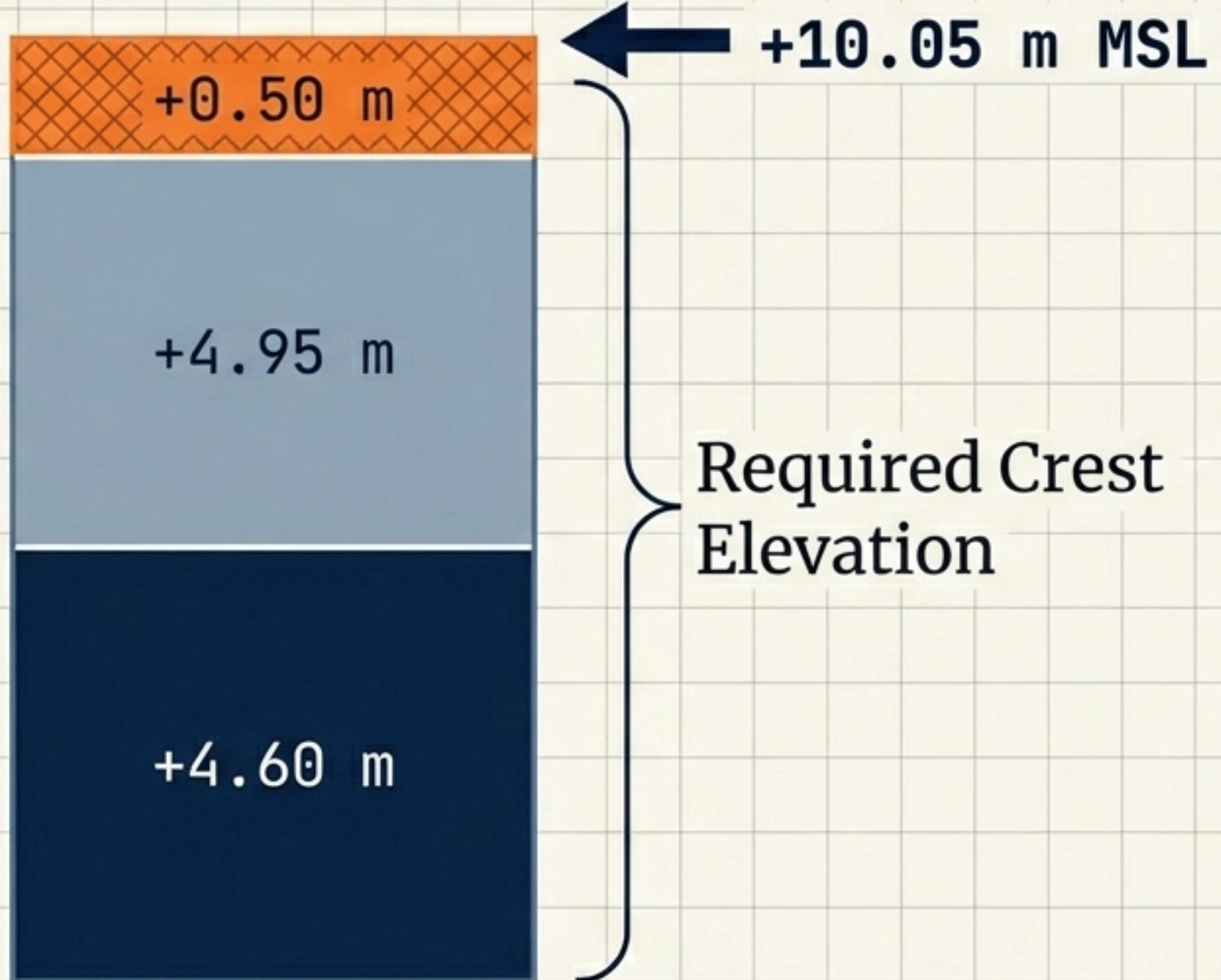
The structure must be built to 10.05m above Mean Sea Level to safely contain the run-up.
