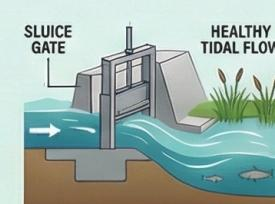
Modern gates can be installed in levees to restore healthy tidal flow to wetlands.
